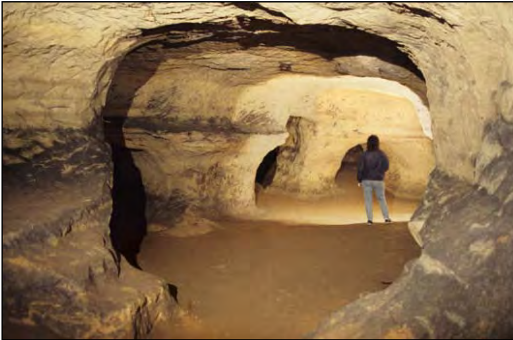
Plate 1 (top left). In the heart of Rouse's sand mine pillars provide stable roof support and some galleries have been broken out to double height (all photos by Tony Waltham).
